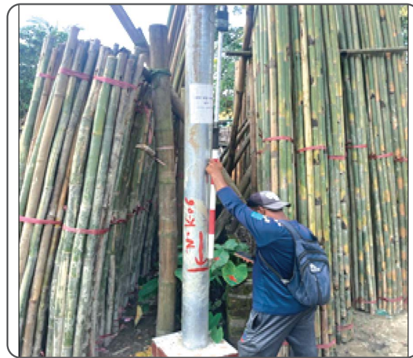
Figure: Interview Survey at Selected Location and Marking of Flood Level by RTK
