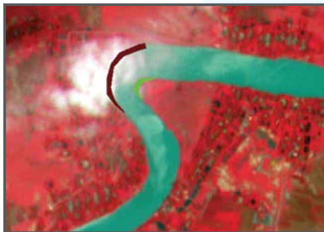
Satellite Image analysis from 2016-2022 at Jalalpur at Kushiya River Right Bank shows erosion and deposition (Brown: Erosion, Green: Deposition)
